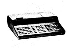
The 9815A calculator is well suited to a variety of applications; acting either as a stand alone calculator or as a controller in a measurement system.
